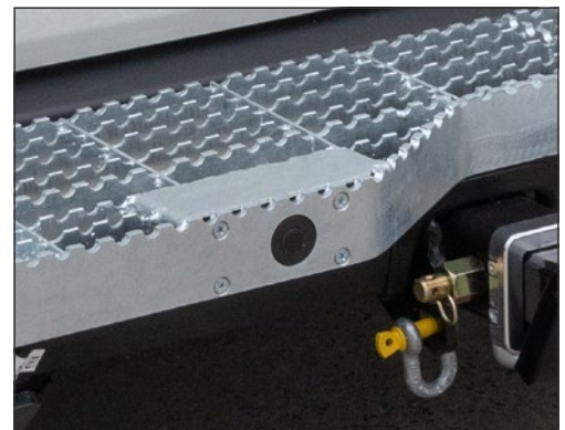
Sensors relocated to the Step
