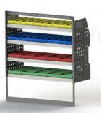
ADJ02-B SPEC-R Unit Size: 1080mm w x 1220mm h End panels: Standard Panel Left, Special Right No. of shelves: 4 Shelf Depth: 310mm (Row 1), 410mm (Rows 2 & 4), 350mm (Row 3) Plastic Bins: 10 x PBC 3.0, 10 x PBC 4.0, 5 x PBC 6.0, 5 x PBC 8.0
