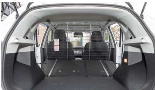
Cargo Barrier Installed behind 1st Row of Seating
