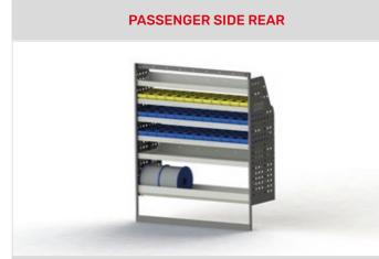
ADJ80-W Unit Size: 1260mm w x 1490mm h End panels: 1200mm High Panels No. of shelves: 5 (1 x Cable Shelf, 1 x Bottom Bar) Shelf Depth: 240mm (Row 1), 310mm (Row 2), 410mm (Rows 3-7) Plastic Bins: 12 x PBC 3.0, 24 x PBC 4.0
