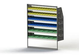
ADJ29-Q Unit Size: 1260mm w x 1760mm h End panels: Standard Panels No. of shelves: 6 Shelf Depth: 310mm (Rows 1 - 2), 410mm (Rows 3 -6) Plastic Bins: 24 x PBC 3.0, 24 x PBC 4.0, 12 x PBC 8.0
